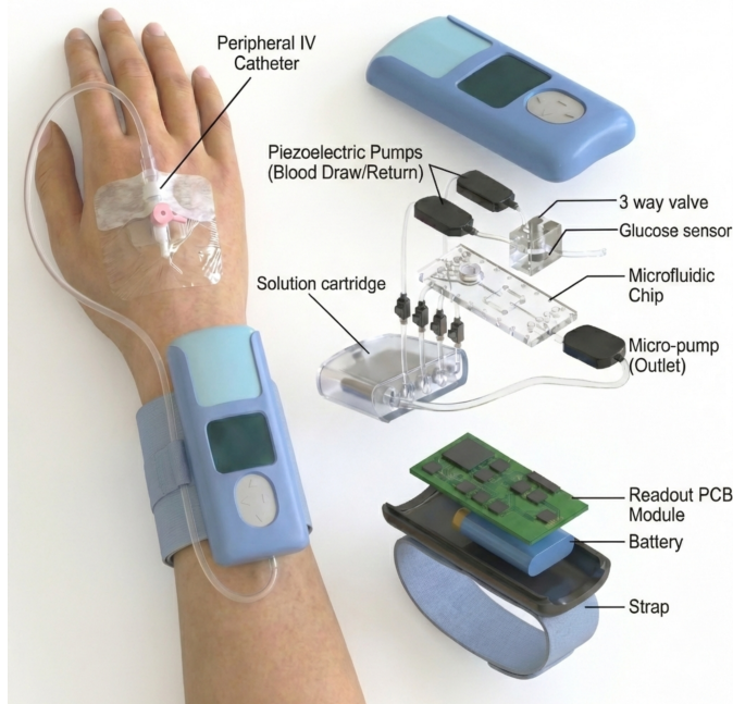
Fig. 1. Conceptual illustration of the proposed automated IV cannula-based blood glucose monitoring system. The graphic was rendered with the assistance of Google Gemini.
